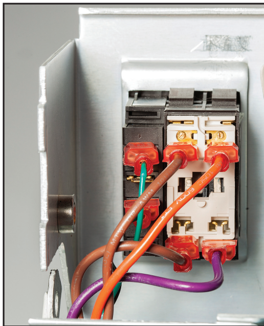
Fig 8-25 Placement of AC Breaker Harness Connections
