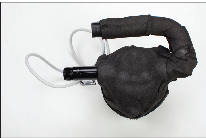
Fig 8-54 Flowmeter with arrow indicating direction of flow; same direction as Circulation Pump outlet
