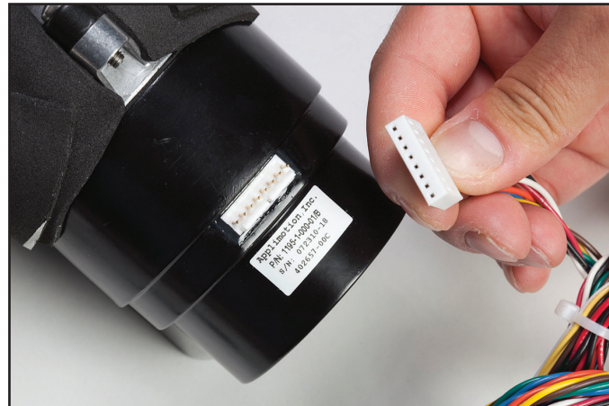
Fig 8-46 Illustration of pump connector prior to being connected (above), connected but seated incorrectly with one pin exposed (below left), and seated correctly (below right)
