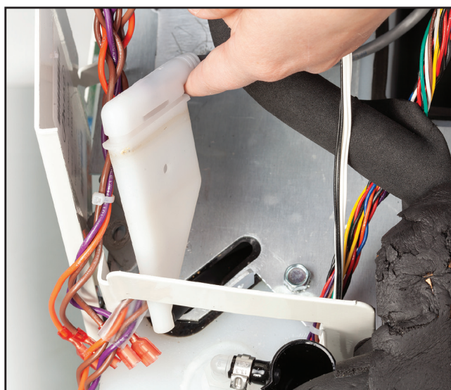
Fig 8-30 Remove Level Sensor and sheath from tank
