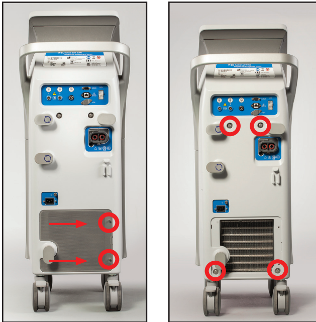
Fig 8-10 Back Panel with removal of screen filter and screws
