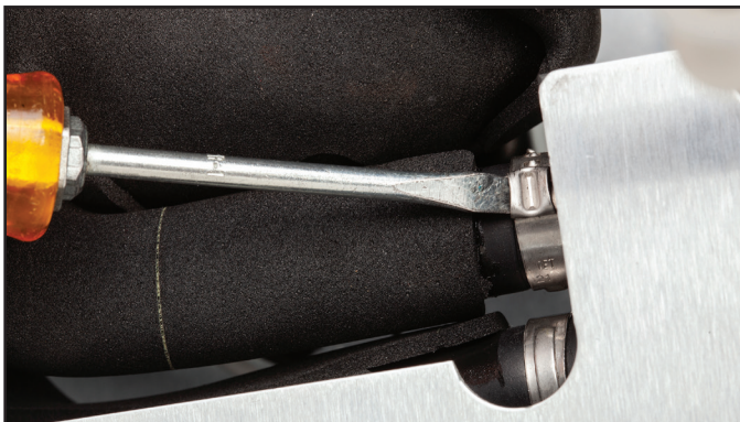
Fig 8-47 loosen the hose clamp that secures tubing to manifold
